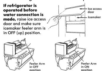
When water supply has been connected to icemaker, move feeler arm to ON (down) position.
